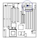
EICA CPU Fan Connector: EICA
