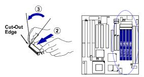
**NOTE**: SIMMs in each bank must be of the same type; and the BIOS automatically configures the memory size.
