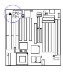
**Power Supply Type Selection: PWR**This jumper allows you to select your power supply type: an AT power supply or remote power supply. Please read CN5 in page 31 of this chapter when your system uses an ATX power supply.
