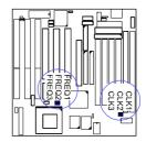
*CPU to Bus Frequency Ratio: FREQ1, FREQ2, FREQ3*These three jumpers are used in combination to decide the ratio of the internal frequency of the CPU to the bus clock.
