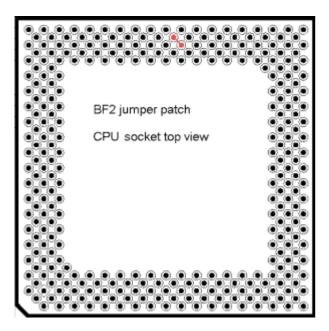
I have selected a bus frequency of 75 Mhz and a multiplier of 5.0 (i.e. 375 Mhz). 5.5 would also work, but the CPU gets very hot then, so you would perhaps need an extra cooler.
