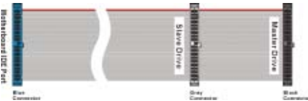
Figure 2-9. Ultra DMA 66 Ribbon Cable Outline
