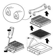
2. Push the lever on the processor socket down and out until it pull up freely. Lift the lever until it stands straight up freely. Lift the lever until it stands straight up. Remove the processor from the socket. Do not touch or bend the pins.
