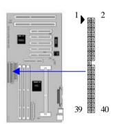
This connector supports two primary channel IDE devices via a ribbon cable. When two IDE devices are installed using the primary IDE connector, make sure that the second IDE device is set to slave mode as indicated in the device's manual.
