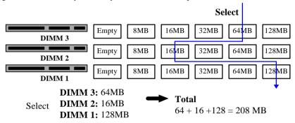
To select 1 out of 6 items (empty, 8MB, 16MB, 32MB, 64MB, 128MB) in DIMM3. Then, repeat again in DIMM2, DIMM1 to go through your own path.
