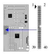
This connector supports two secondary channel IDE devices as well as the 120MB Floppy drives via a ribbon cable. When two IDE devices are installed using the secondary IDE connector, make sure that the second IDE device is adjusted to slave mode as instructed in the device's manual.
