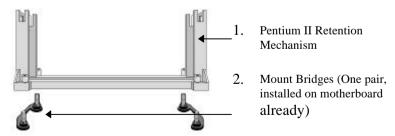
In your Packaging, one Pentium II Retention Mechanism is attached and one pair of Mount Bridges is installed on the motherboard.
