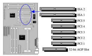
PCI expansion slots and one 32-bit AGP slot as shown above.
