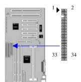
The FDC sub-system can control three types of floppy drives (1.2, 1.44 and 2.88MB) or compatible tape drives. The connection to the floppy drive is via a header (J19). The floppy disk interface includes 48mA drivers and inputs on the drive interface.
