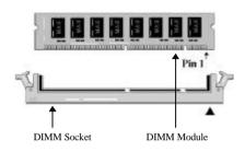
Step 3: After inserting the DIMM module completely into the socket, push up on the
