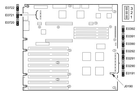
Figure B–1 Location of System Board Jumpers
