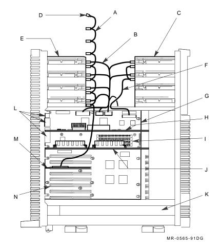
Figure 1–3 System Cabinet, Internal View
