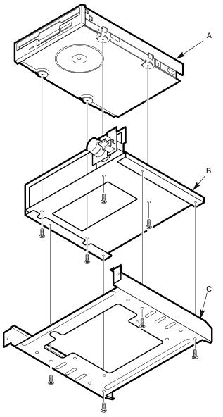
Figure 4–13 RX23 3.5-Inch Diskette Drive Removal (Part 2 of 2)
