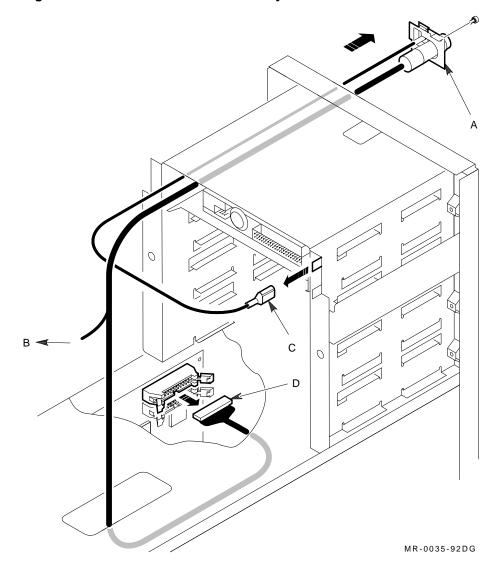
Figure 4–26 Front Panel Wire Assembly Removal
