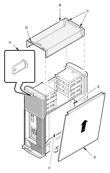
Figure 4–1 System Cover and Side Panel Removal
