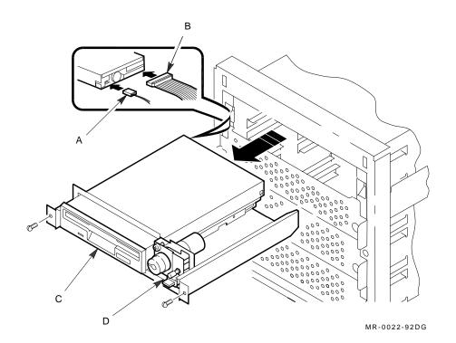
Figure 4–12 RX23 3.5-Inch Diskette Drive Removal (Part 1 of 2)
