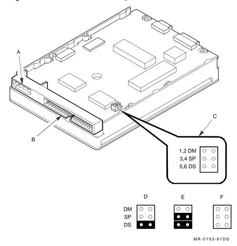
Figure 4–23 105 MB IDE Drive Jumper Locations
