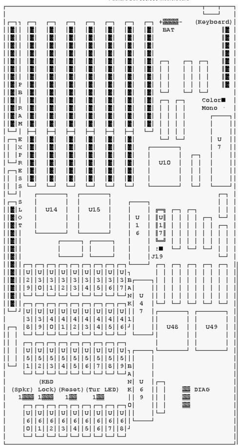
NOTE: Holds 1MB of RAM (256 x 1 chips), arranged in four rows of nine chips per row (8 bits of RAM and 1 parity bit.) The CMOS backup battery is a removable AT style battery.
