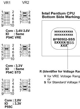
XXXXXXXXXX BP80502-SSS SXXXX/<u>R</u>SS XXX R (Identifier for Voltage Range) : V for VRE Voltage Range or **S** for Standard Voltage Range
