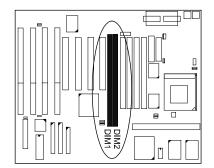
2. Carefully insert the DIMM straight down onto the DIMM slot with both hands until the clips on the ends of the slot close up to hold the DIMM in place.
