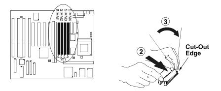
**NOTE :** SIMMs in each bank must be of the same type; and the BIOS automatically configures the memory size.
