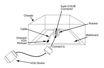
The serial port COM2 on this mainboard is designed to be a SIR compliant port. If you wish to install the SIR connection feature, you need to adjust the BIOS option for high-speed performance.
