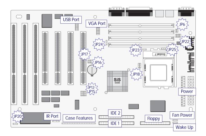
Jumper & Connectors The illustration above shows the location of the jumpers, port and other connectors on the P5SJ–A mainboard.
