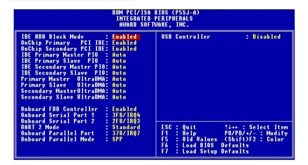
CMOS Setup Utility – Integrated Peripherals This section of the setup utility configures the IDE and Floppy controllers and the settings for the external ports This section enables and configures the optional USB and Infrared features.
