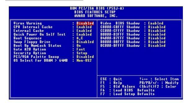
CMOS Setup Utility – BIOS Features Setup This section of the setup utility allows you to configure some system features including Virus Warning, Boot Sequence and Security Option. Virus Warning –
