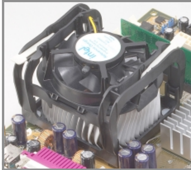
Figure 2-11 Fan and Retention Mechanism Installed and Locked
