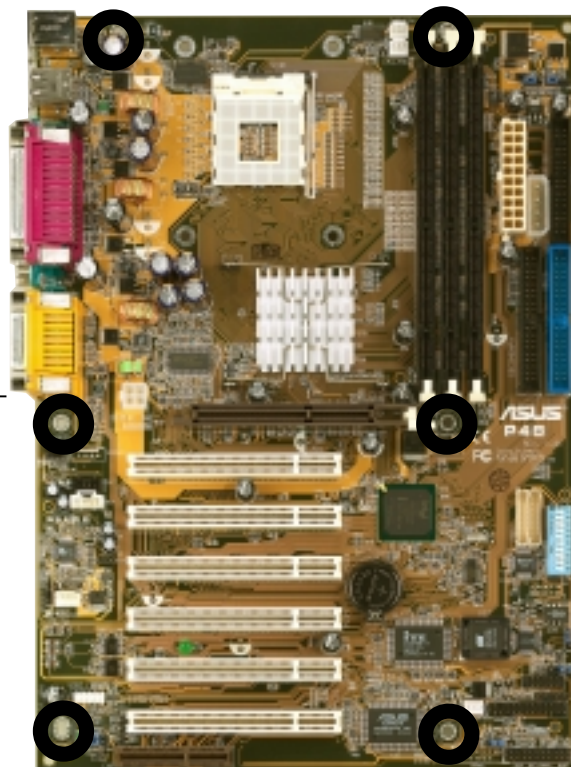
Figure 2-1 Motherboard placement and screw holes
