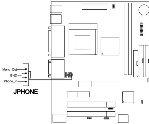
Mono\_Out is connected to the Modem Speaker Out connector.
