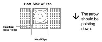
In case the metal clips are detached from the Heat Sink, re-attach them. Look for the arrow on the metal clip. This arrow should be pointing down and aligned with the Heat Sink Support Base Holder.
