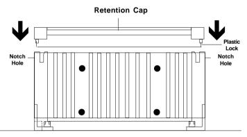
Lock the processor by putting the Retention Cap provided. Take note of the two plastic lock at the side of the Retention Cap. This two plastic lock should be aligned properly into the Retention Mechanism notch hole.
