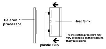
Push down the plastic clips, so that they are in line with the hole on the processor. Check for perfect fit.
