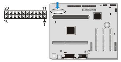
This connector supports a standard ATX power supply. When connecting, make sure the lock key matches the hook attached on a power supply cable. The power cord should be unplugged when you connect it.
