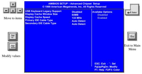
Figure 4: Advanced Chipset Features Setup Menu
