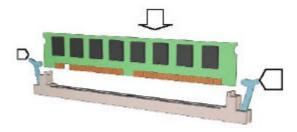
Be careful not to misfit the DIMM Module into DIMM sockets in wrong direction. This module can be inserted into the socket only one way. Please note the "\( \Lambda \)" for pin 1 location. To release the memory module, push both latches down and carefully rock the module forward and backward while slowly lifting it upward.
