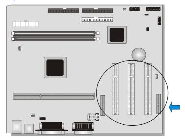
This motherboard contains 5 expansion slots (including one shared PCI/LVR) onboard. Three 32-bit PCI expansion slots, one AMR slot and one LVR slot as shown above.
