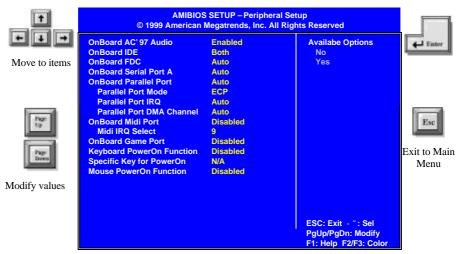
Figure 5: Integrated Peripherals Setup Menu
