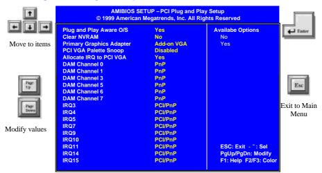
Figure 7: PCI/ Plug and Play Configuration Setup Menu
