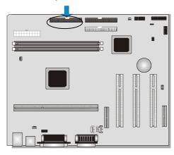
The FDC sub-system can control three types of floppy drives (1.2, 1.44 and 2.88MB) or compatible tape drives. The connection to the floppy drive is via a header. The floppy disk interface includes 48mA drivers and inputs on the drive interface.
