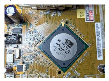
The heatsink is glued to the chip with some pink filth, it's almost impossible to remove it without harm to the NB. Everything gets better if you make radiator hot (45-50 degrees C), then it can be removed safely. I used the same heatsink with good thermal compound.
