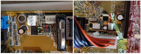
3) Absent RAM slot is soldered to the motherboard, since the voltage for DDR is tested on the missed pins, and it's OK. I supposed, that the missing slot is working and only needs to be soldered on.
