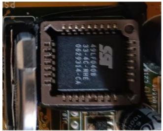
The original BIOS chip is SST 49LF040, this one is 49LF040B, it's fully compatible.
