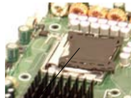
Plastic cap is released from the load plate if CPU properly installed.
