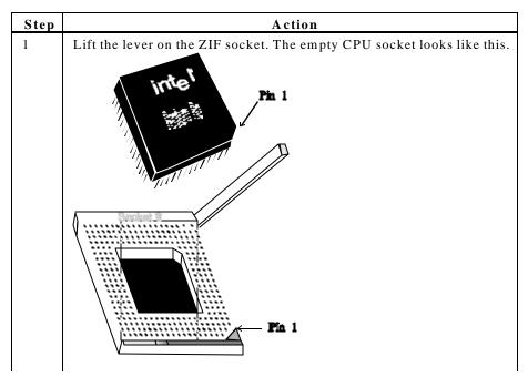
2 Check for bent pins on the CPU. Gently straighten any bent pins with pliers. Place the CPU in the middle of the socket, as shown below. Make sure that pin 1 of the CPU is aligned with pin 1 of the socket. Make sure you are properly grounded while handling the CPU.
