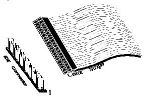
J12 is a 40 – pin dual – inline berg that connects an IDE drive to the primary onboard IDE connector. This motherboard supports IDE Modes 0, 1, 2, 3, and 4, IDE prefetch, LBA (Logical Block Address) mode, high capacity drives (over 528 MB), 32 – bit data transfer, and fast IDE transfer. These IDE features are configured in Peripheral Setup in the WINBIOS Setup utility.
