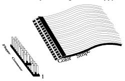
The motherboard supports up to two 720 KB, 1.44 MB, or 2.88 MB  $3\frac{1}{2}$ " drives and 360 KB and 1.2 MB  $5\frac{1}{4}$ " drives. The connecting cable is a 34 – pin ribbon connector with two 34 – pin edge connectors for attaching the floppy disk drives. There is a small twist in the cable between the floppy connectors. The last (end) connector should be connected to floppy drive A:.
