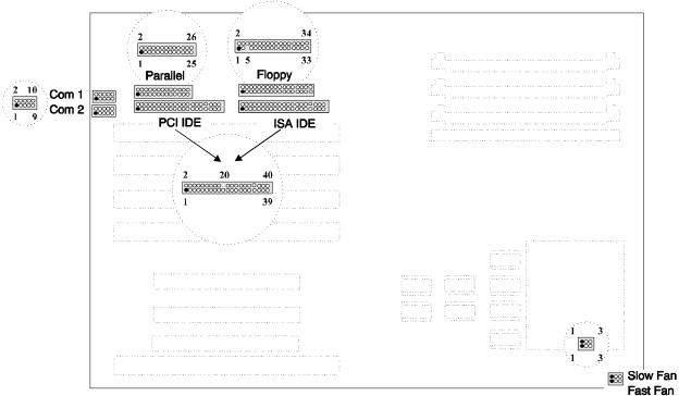
Figure 4. I/O Connections
