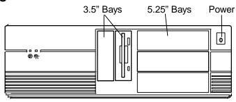
Figure 5: Premiere/PCI Expandable Desktop Front Panel
