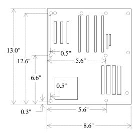
Figure 1. Premiere/PCI Baby-AT Motherboard dimensions.
