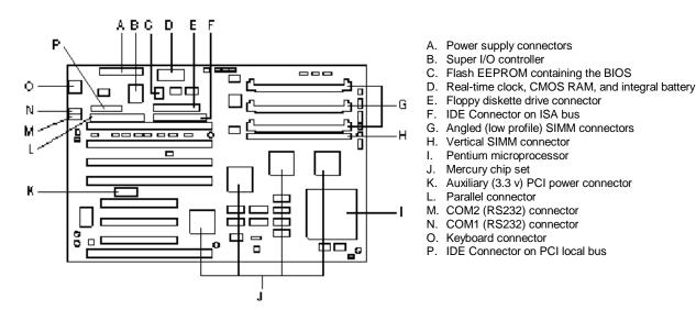
Figure 2. Premiere/PCI Baby-AT Motherboard components
