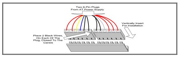
**AT Power Connector Installation**
