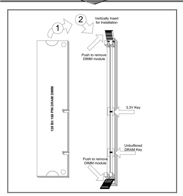
168-Pin SDRAM Module Installation Diagram
