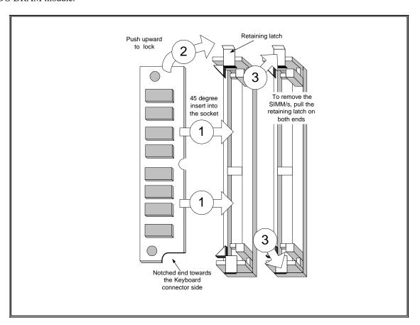
**SIMM Module Installation Diagram**
