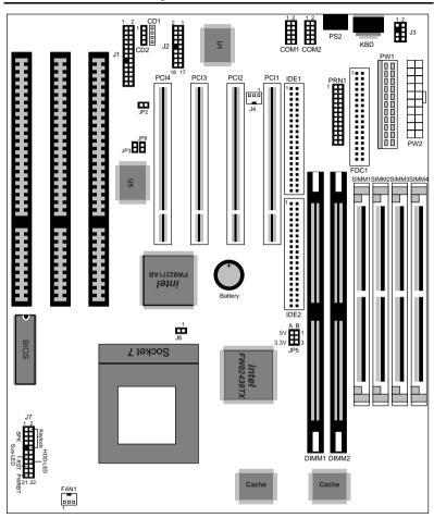
Figure 2–1. Mainboard Component Locations
