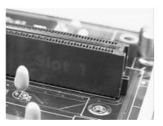
Then carefully line up the key notch on the Retention Module with the key pin on the Pentium II Slot. (The key pin on the Pentium II Slot indicates the correct orientation of the CPU.)
