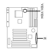
\*For Cyrix settings, please refer to the CPU Voltage table. For all CPUs, please refer to the BUS Settings and CPU Speed Settings tables. VC1 and VC2 should be set to OFF for Pentium non-MMX CPUs, and ON for all other CPUs.
