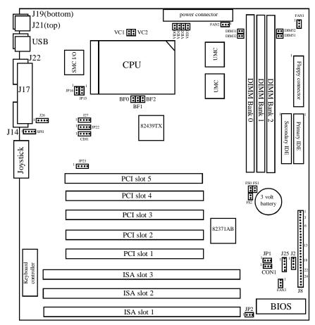
The following jumpers and connectors are optional, and will only be present if your board has the Ensoniq sound chip installed: J26, J27, JP22, JP23, CDI1, and Joystick.
