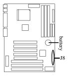
battery is 10 years, but if yours is running low, you will need to replace it with a new 3V lithium battery (Duracell DL2032).
