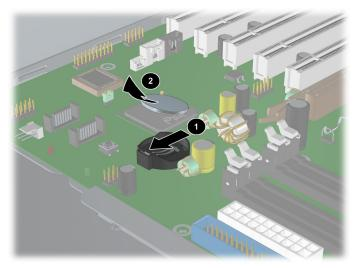
To install the battery slide the battery back in until it snaps back into place.
