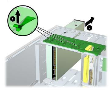
3. After pulling the drive ① out, remove the four guide screws ② from the drive as shown in the following illustration.
