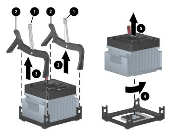
To replace the heatsink assembly, reverse the previous steps. New thermal grease must be applied between the heatsink and processor.
