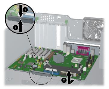
To replace the system board, slide the board back in and lay it down until the release tab snaps it back into place. Re-install all cards and reconnect all cables.
