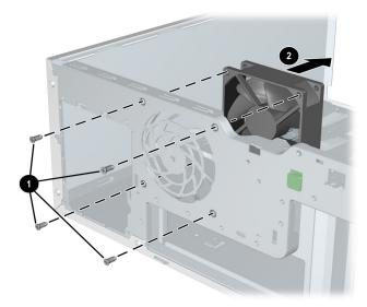
3. Slide the fan **2** toward the front of the unit and remove it.
