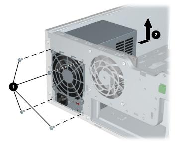
4. Slide the power supply **2** toward the front and lift up to remove it from the chassis. To install the power supply, reverse the previous steps.
