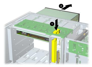
3. After pulling the drive ① out, remove the four guide screws ② from the drive as shown in the following illustration.
