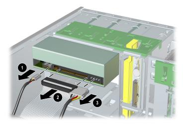
2. After the front bezel and bezel blanks have been removed, press down on the yellow drivelock as shown in the following illustration. As you press on the yellow drivelock ●, gently slide the drive ② out of the chassis.
