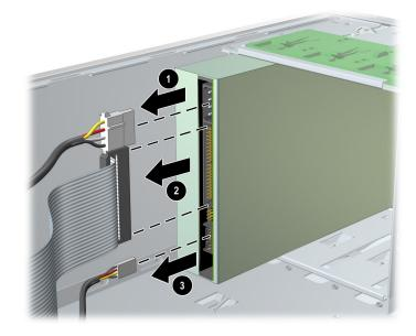
2. After the front bezel and bezel blanks have been removed, lift the green drivelock release lever **1** and gently slide the drive **2** out of the chassis.
