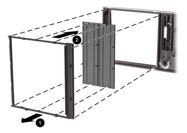
NOTE: The bezel blanks are keyed to assist you in replacing the blanks.
