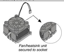
Connect the CPU Cooling Fan power cable connector to the CPUFAN connector.
