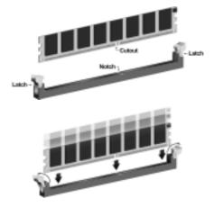
Install the DIMM module into the slot and press it firmly down until it seats correctly. The slot latches are levered upwards and latch on to the edges of the DIMM.
