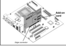
Secure the metal bracket of the card to the system case with a screw.
