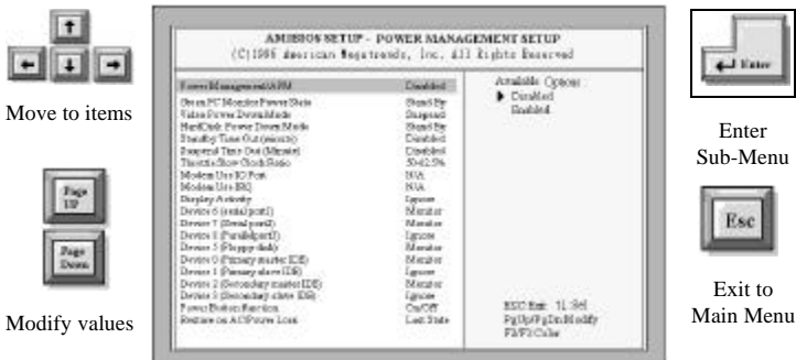
Figure 5 : POWER MANAGEMENT SETUP
