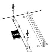
4. Install two Retention Mechanism Attachment Mounts on the board
