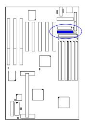
*Front Panel Block Connector: F\_PNL* This block connector includes: PW\_LED, KB\_LOCK, TB\_LED, SP\_SW, SPK, SP\_LED, IDE\_LED, RPW\_SW, and RST connectors.
