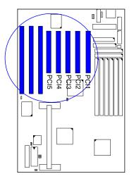
This section describes how to connect an expansion card to one of your system's expansion slots. Expansion cards are printed circuit boards that, when connected to the mainboard, increase the capabilities of your system. For example, expansion cards can provide video and sound capabilities.
