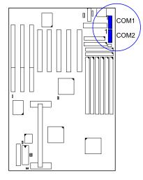
These two 10-pin male connectors allow you to connect devices that take serial ports, such as a serial mouse or a modem. The COM2 Port on the KN-6000 mainboard can also be used as another IR Port. Usually, your serial mouse is attached to COM1. Your modem is linked to COM2. When you do not use the modem, you can set the BIOS to let COM2 be an IR port to save a dedicated SIR port.
