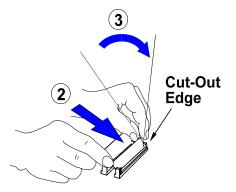
3. Swing each SIMM into its upright, locked position. When locking a SIMM in place, push on each end of the SIMM - do not push in the middle, as shown above.
