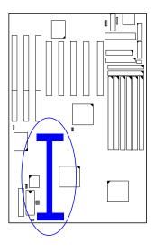
2. Locate the Heatsink Support Base on the mainboard.
