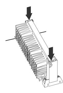
10. Hook the Heatsink Top Support to the Heatsink Support Base to affix the CPU module.
