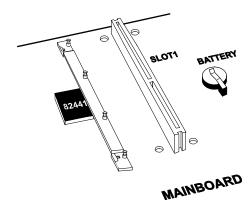
3. Affix it by inserting one "T"-shaped plastic plugs into the hole on each end.
