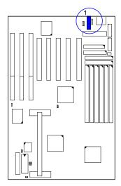
This 10-pin male connector is used for connecting to the infrared (SIR) port and allows transmission of data to another system which also supports the SIR feature.
