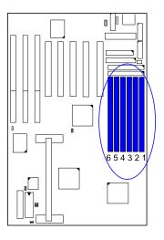
**NOTE :** SIMMs in each bank must be of the same type; and the BIOS automatically configures the memory size.
