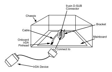
The serial port COM2 on this mainboard is designed to be a SIR compliant port. If you wish to install the SIR connection feature, you need to adjust the BIOS option for high-speed performance. Please read page 55 of this manual.
