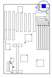
This 5-pin female connector is used for your 101-key enhanced keyboard or 106-key Windows 95 keyboard.
