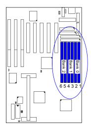
The DRAM module installation must be in pairs of the same size for each bank. The minimum size of SIMM for each SIMM slot is 4MB; the maximum is 128MB\*. Each bank, not SIMM slot, can be leaved empty.
