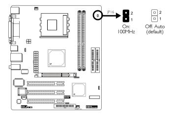
This jumper is used to select the front side bus of the CPU installed on the system board. The default setting is Auto. The system will run according to the front side bus of the CPU installed on the system board. You can also set the FSB fixed at IOOMHz by setting IP16 to On.
