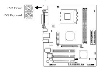
The system board is equipped with an onboard PS/2 mouse (Green) and PS/2 keyboard (Purple) ports - both at location CNI of the system board. The PS/2 mouse port uses IRQ12. If a mouse is not connected to this port, the system will reserve IRQ12 for other expansion cards.
