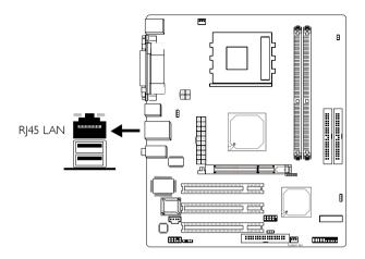
The system board is equipped with an onboard RJ45 fast-ethernet LAN port at location CN6 of the system board. It allows the system board to connect to a local area network by means of a network hub.
