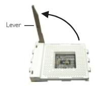
5. Position the CPU above the socket then align the gold mark on the corner of the CPU (designated as pin I) with pin I of the socket.
