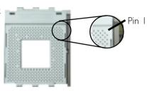
6. Insert the CPU into the socket until it is seated in place. The CPU will fit in only one orientation and can easily be inserted without exerting any force.
