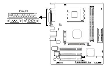
The system board has a standard parallel port (Burgundy) at location CN7 for interfacing your PC to a parallel printer. It supports SPP, ECP and EPP.
