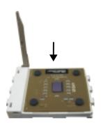
7. Once the CPU is in place, push down the lever to lock the socket. The lever should click on the side tab to indicate that the CPU is completely secured in the socket.
