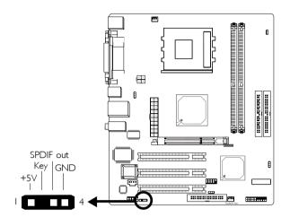
The S/PDIF-out connector (J3) is used to connect external S/PDIF port. The S/PDIF-out port may be mounted on a card-edge bracket. Install the card-edge bracket to the system chassis then connect the audio cable connector to J3. Make sure pin I of the audio cable connector is aligned with pin I of J3.
