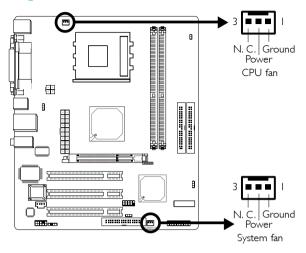
Connect the CPU fan's cable connector to the CPU fan connector (J4) on the system board. The system fan connector (J8) is used to connect an additional cooling fan. The cooling fans will provide adequate airflow throughout the chassis to prevent overheating the CPU and system board components.
