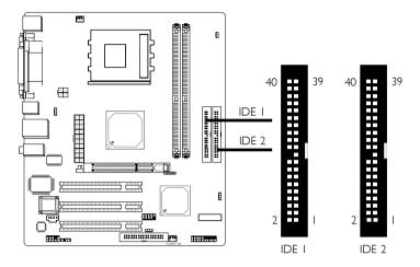
The system board is equipped with two shrouded PCI IDE headers that will interface four Enhanced IDE (Integrated Drive Electronics) disk drives. To prevent improper IDE cable installation, each shrouded PCI IDE header has a keying mechanism. The 40-pin connector on the IDE cable can be placed into the header only if pin I of the connector is aligned with pin I of the header.
