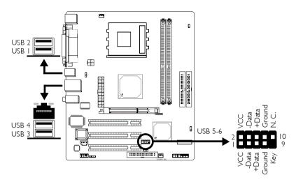
Four onboard USB 2.0/1.1 ports (Black) are at locations CN5 (USB 1-2) and CN6 (USB 3-4) of the system board.
