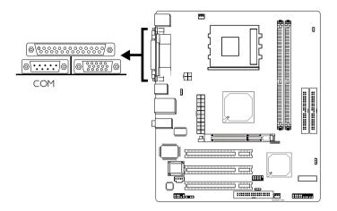
The system board is equipped with an onboard serial port (Teal/Turquoise) at location CN4 of the system board. It is a RS-232C asynchronous communication port with I6C550A-compatible UART that can be used with a modem, serial printer, remote display terminal or other serial devices.
