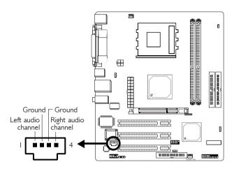
The CD-in (J2) connector is used to receive audio from a CD-ROM drive, TV tuner or MPEG card.
