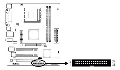
The system board is equipped with a shrouded floppy disk drive connector for connecting a standard floppy disk drive. To prevent improper floppy cable installation, the shrouded floppy disk header has a keying mechanism. The 34-pin connector on the floppy cable can be placed into the header only if pin I of the connector is aligned with pin I of the header.
