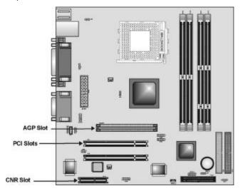
AGP Slot The 4xAGP slot is used to install a graphics adapter that supports the
