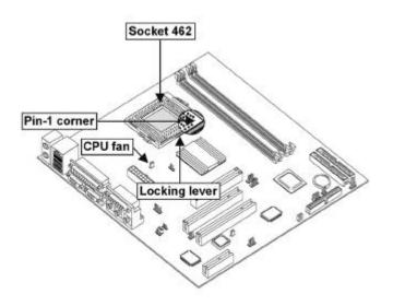
**Note:** The pin-1 corner is marked with an arrow **r**
