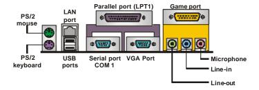
**PS/2 Mouse**Use the upper PS/2 port to connect a PS/2 pointing devices.
