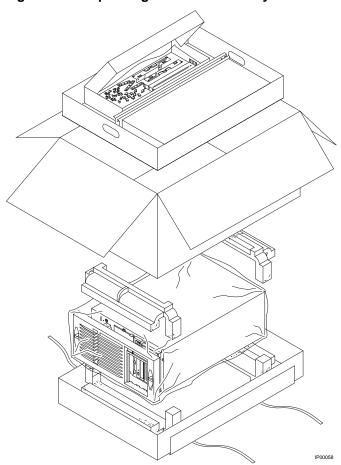
Figure 2-1 Unpacking the Rackmount System
