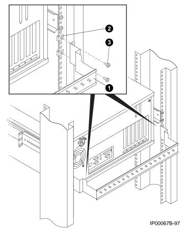
Figure 2-6 Installing the Cable Management Bracket
