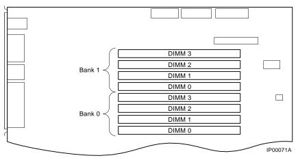
WARNING: Before installing a memory module, turn off all power to the system.
