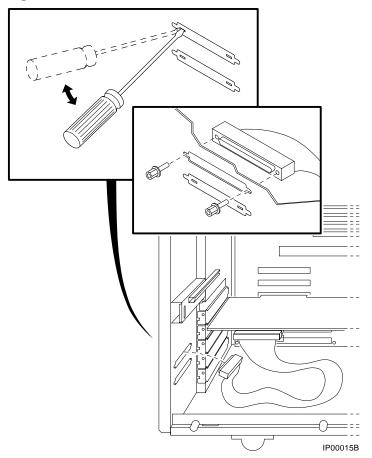
Figure 10-14 Wide SCSI Cable for Breakouts at Rear of Enclosure
