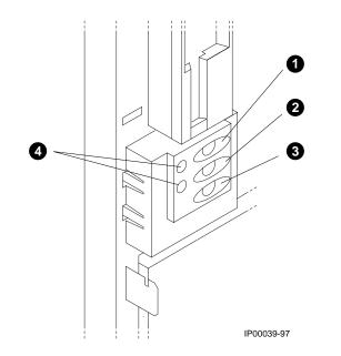
The control panel consists of three pushbutton controls and two LED indicators:
