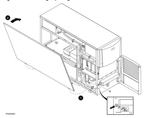
Figure 10-1 Removing/Replacing Side Panel on a Pedestal
