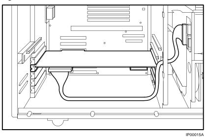
Figure 9-2 RAID Cable for Hard Disk Drives
