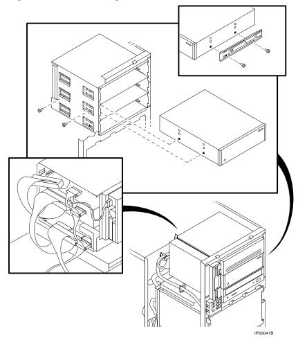
Figure 10-12 Continuing Installation of a 5.25-Inch Device
