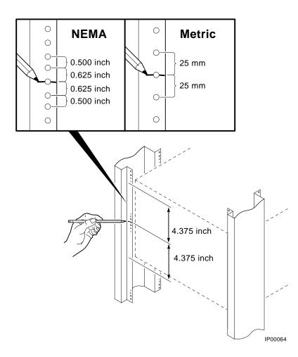
The installation of the rackmount system requires 8.75 inches (5U) of vertical height in the cabinet.
