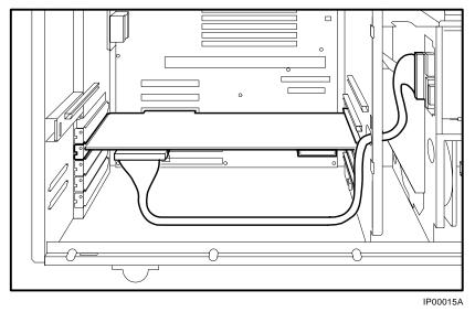
Figure 10-13 RAID/SCSI Cable for Internal Disk Drive Backplane
