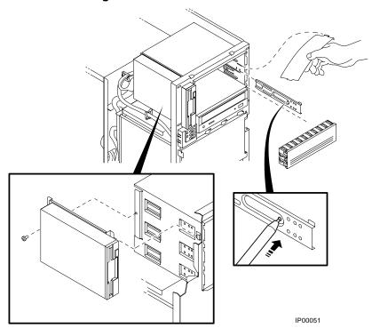
Figure 10-11 Installing a 5.25-Inch Device
