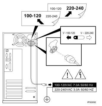
*NOTE: Current ratings are maximum with a fully loaded system and do not include a monitor or terminal.*
