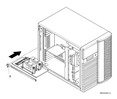
Figure 5-4. Installing the Processor Module
