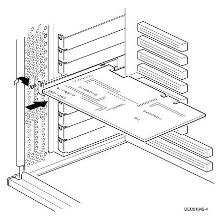
Figure 8-3. Installing an Expansion Board
