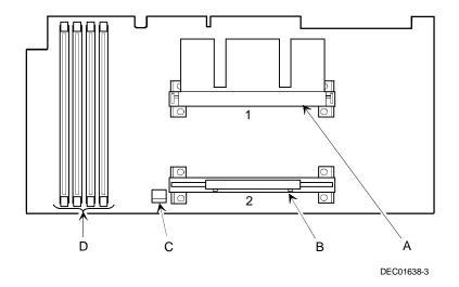
Figure 3-10. Processor Module Component Locations
