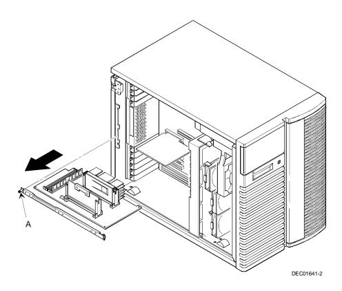
Figure 5-1. Removing the Processor Module
