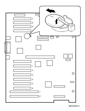
Figure 3-12. Replacing the Server Battery/RTC
