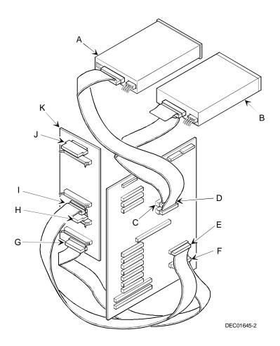
Figure 9-2. Split Backplane Configuration Using Onboard SCSI Controllers
