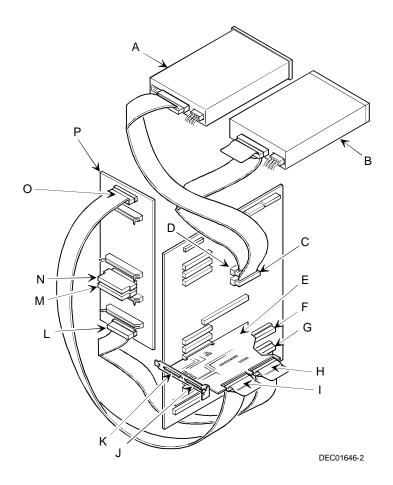
Figure 9-3. Split Backplane Configuration Using Two Channel RAID Adapter
