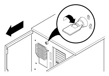
Figure 10-2. Left and Right Side Panel Lock
