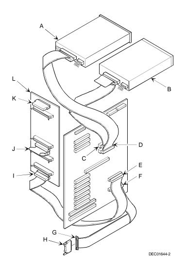
Figure 9-1. Single Backplane Configuration Using an Onboard SCSI Controller
