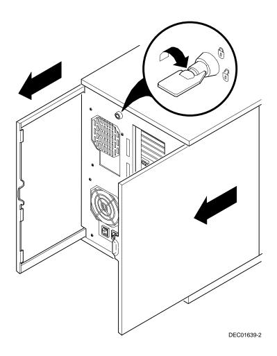
Figure 3-2. Unlocking and Removing the Side Panels
