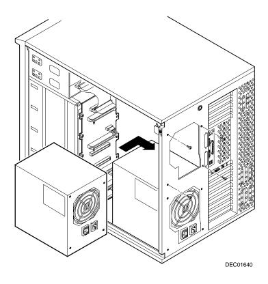
Figure 3-13. Adding A Second Power Supply
