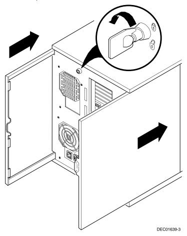
Figure 3-3. Installing the Side Panels
