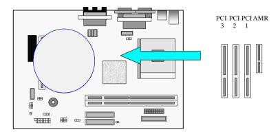
This motherboard contains 4 expansion slots onboard. Three 32-bit PCI expansion slots and one AMR slot as shown above.
