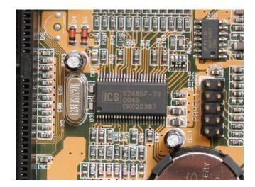
The familiar ICS 9248-39 is used as the clock generator IC. Standard stone of this era from 66 to 150MHz. The clock can be changed by software.
