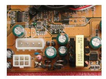
Power supplies that generate 5V and 3.3V are still alive. The compatibility with the BKi810 is maintained together with the original 6-pin 12V power supply, but it is unavoidable that the compatibility with the ATX standard will drop instead.
