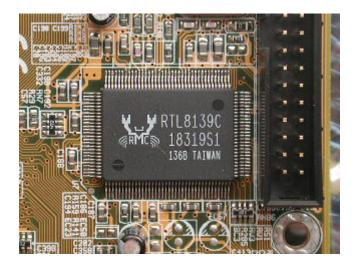
The LAN chip has changed from DM9102F to the general Realtek RTL8139C. The CPU usage is a little high, but there is no particular problem with stability. Much better than a product that seems to be stuck with driver updates.
