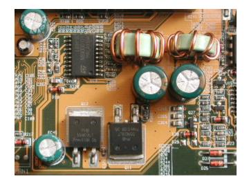
VRM has been changed to a general synchronous rectification method. Is from V7.x of BKi810, but the VRM controller is L6911B instead of HIP6004B adopted in BKi810 (V7.x). These are compatible chips including RT9224 (pin compatible and can be replaced as it is) ). I'm looking forward to the comparison with the discrete VRM of KA7500B. PHB55N03LT is used for the up and down switch. It is a standard
