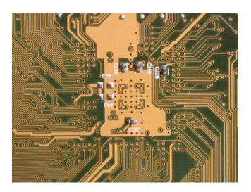
The north bridge is FSB 133MHz and has VGA built-in, so it is relatively strictly DC. It works without it, but if the cause is unknown, this may be the cause, so it's a big enemy. If the video with built-in chipset is not working well with high FSB, this may help. Other than that, there is no meander wiring like DDR, so it can not be said that it is a particularly difficult chip.
