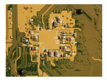
DC on the back of the CPU. Is it unstable for C3 to say that ECS, which is famous for stingy, is DC so tightly? However, since this CPU is a BGA package, it cannot be attached inside the socket, so it may be natural to attach it to the back.
