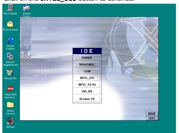
When the IDE \ INTEL\_815 box appears on your screen, click on the INTEL\_R&HIPSET\_SOFTWARE\_INS to install the IDE plug and play information files into your system.
