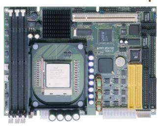
The HS-4700 is an Intel® 82845 chipset-based board designed for PCI Bus PGA 478 Intel® Pentium® 4 1.2~2.2GHz(400MHz FSB) CPU compatibility. These features combine and make the HS-4700 an ideal all-in-one industrial single board computer. Additional features include an enhanced I/O with CRT/Panel, Dual LAN, Audio and 4COM ports interface.
