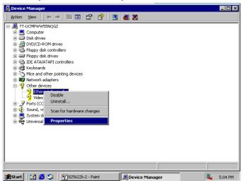
4. Once the **Ethernet Controller Properties** screen pops on the screen, click on the **Update Driver** ... button to launch the **Update Device Driver Wizard** screen. Once the **Upgrade Device Driver Wizard** screen pops on the screen, click **Update Driver** ... to launch the Win 2000 driver installation program.
