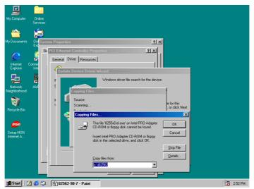
With the Utility CD Disk on your CD drive, key in d:\win98\_se\setup\win98 on the blank space below <u>Copy files</u> from: then press the **OK** button.
