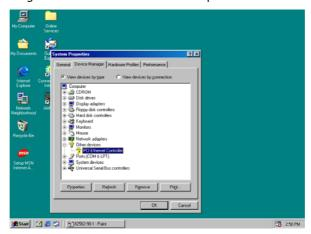
Once the PCI Ethernet Controller Properties screen pops on the screen, click on the Update Driver ... button to launch the Update Device Driver Wizard screen.
