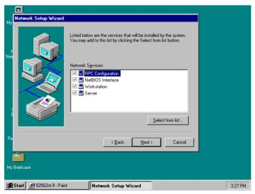
11. The Network Setup Wizard then prompts you that it is ready to install the network components based on your selection. You may start installing by clicking on he <u>Next</u> > button or make modifications on your choices using the < <u>Back</u> button.
