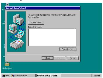
5. When it is done searching for available network drivers, the wizard will show a list and allow you to locate and choose the appropriate Network Adapter. Since the LAN device driver is in the Utility CD Disk, select on Have Disk ... to proceed.
