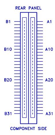
The following figure shows the pin numbering for I/O channel connectors (C-side and D-side).
