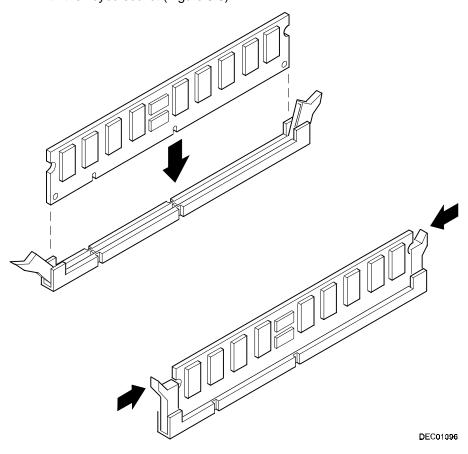
Figure 6-3. Installing a DIMM
