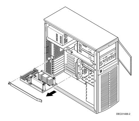
Figure 6-2. Removing a Processor Module
