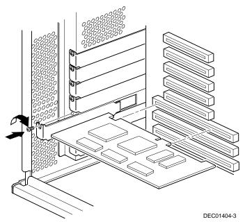
Figure 8-3. Installing an ISA Expansion Board
