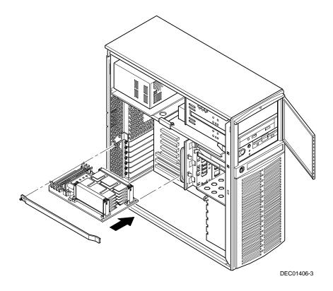
Figure 6-4. Installing a Processor Module
