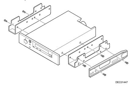
Figure 7-2. Installing Expansion Brackets
