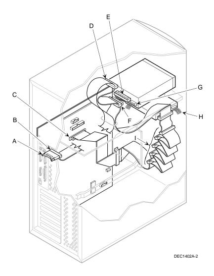
Figure 9-1. Single Channel SCSI Configuration
