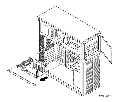
Figure 5-1. Removing a Processor Module
