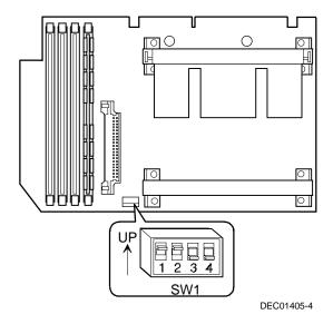
Figure A-2. Pentium II Processor Module Locations
