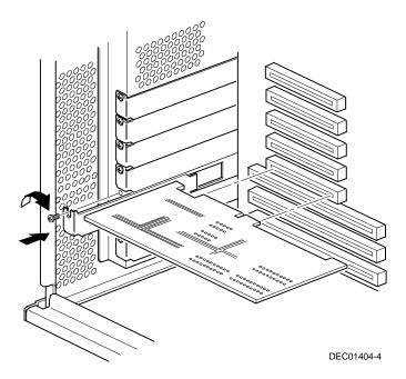
Figure 8-4. Installing a PCI Expansion Board
