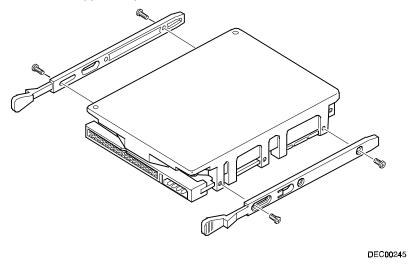
Figure 7-3. Installing Expansion Brackets (Internal Drive Bay)
