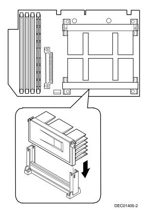
Figure 5-3. Installing the Second Processor
