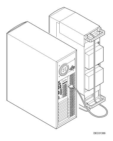
Figure 7-5. Connecting an External SCSI Storage Box
