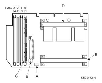
**Figure 3-7. Processor Module Component Locations**
