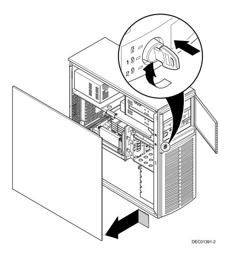
Figure 3-1. Unlocking and Removing the Side Panel
