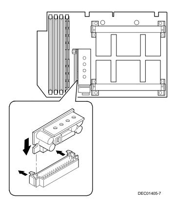
Figure 5-4. Installing the VRM
