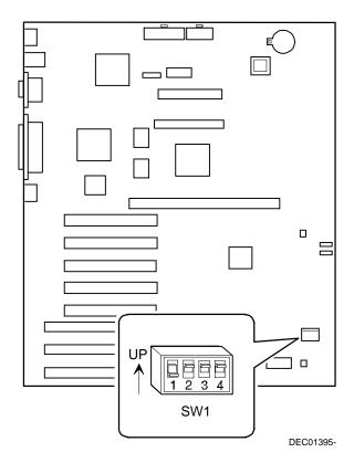
Figure A-1. Main Logic Board Switch Locations
