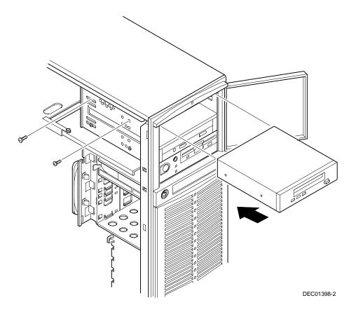
Figure 7-1. Installing a 51/4-Inch Device into the Front Access Drive Bay
