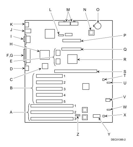
Figure 3-6. Main Logic Board Components and Connectors
