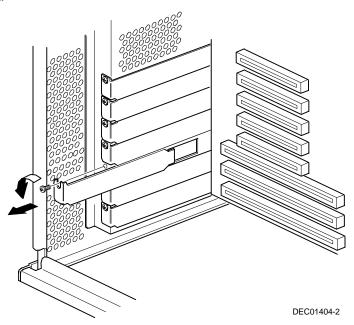
Figure 8-2. Removing a Metal Filler Plate
