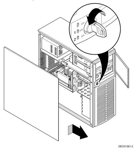
Figure 3-2. Installing the Side Panel
