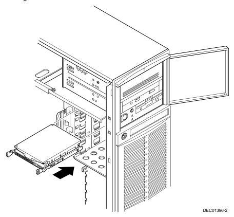
Figure 7-4. Installing a 3½-Inch Device Into the Internal Drive Bay
