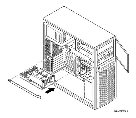
Figure 5-5. Installing the Processor Module
