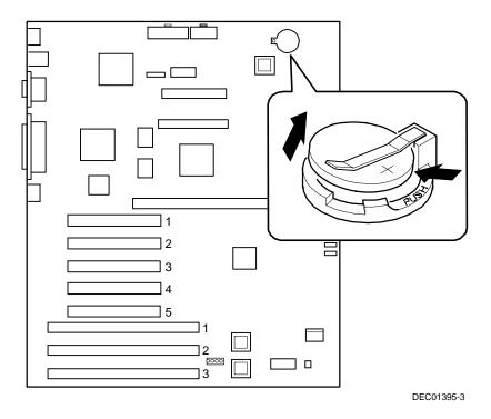
Figure 3-8. Replacing the Battery
