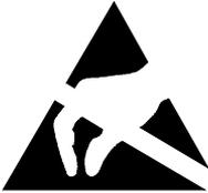
Boards with electrostatic sensitive devices (ESD) are identifiable by the label shown.
