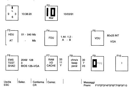
This menu contains all the icons of the BUILT IN SETUP utility, therefore it allows you to configure the system as previously explained.
