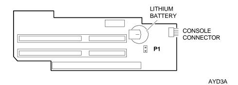
P1 installed: Battery connected
