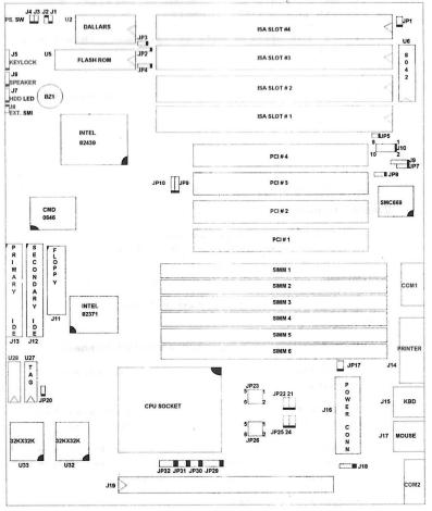
\*Note: PCI slot 4 can not be installed with master card (eg. SCSI, network card).
