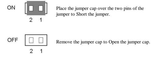
**Note:** To avoid losing jumper caps, attach the removed jumper cap to one of the jumper pins.
