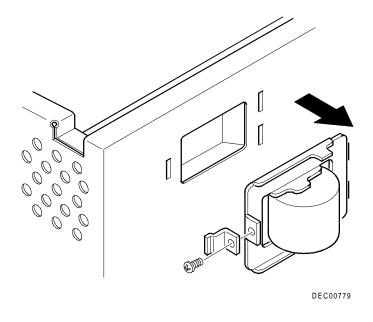
Figure 12-10. Removing and Replacing a Caster
