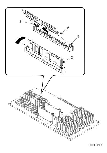
Figure 6-3. Installing a SIMM
