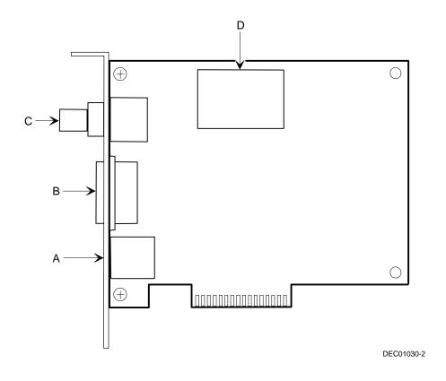
Figure 3-11. Ethernet Daughter Card Components and Connectors
