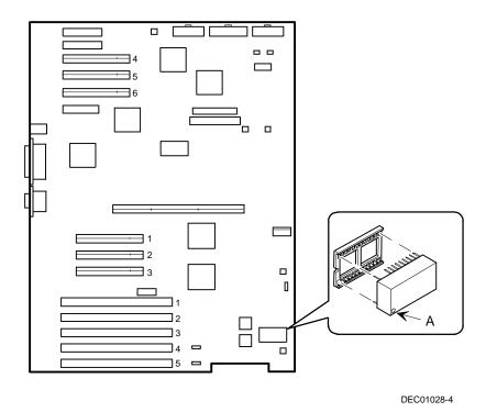
Figure 3-12. Replacing the Server Battery/RTC
