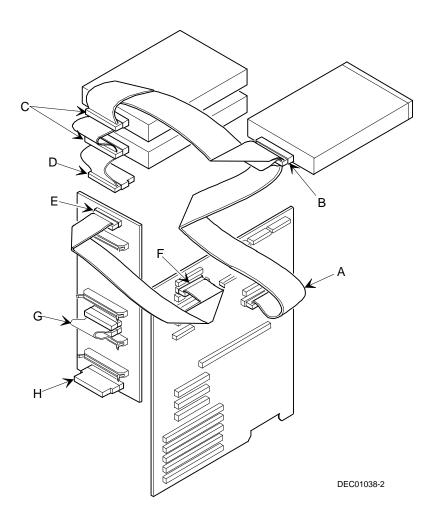
Figure 9-1. Single Backplane SCSI Configuration
