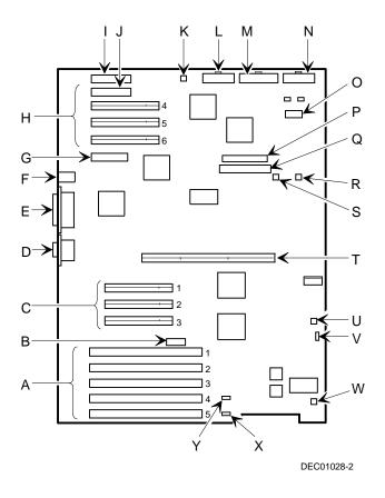
Figure 3-8. Main Logic Board Connectors
