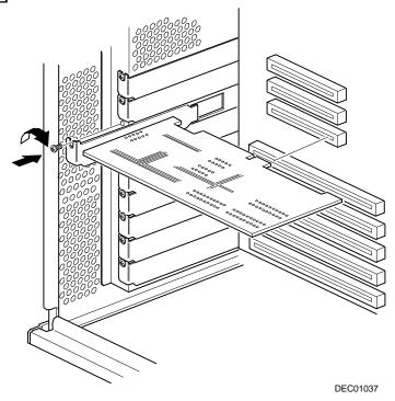
Figure 8-6. Installing a PCI Expansion Board
