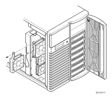
Figure 12-5. Removing and Replacing the Secondary Cooling Fan 2
