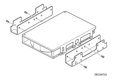
Figure 7-4. Installing Expansion Brackets
