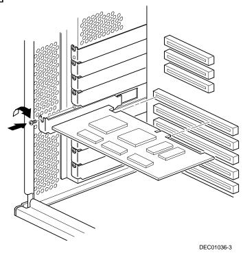
Figure 8-4. Installing an ISA Expansion Board
