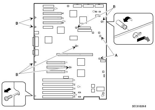
Figure 12-8. Removing and Replacing the Main Logic Board
