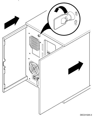
Figure 3-3. Installing the Side Panels
