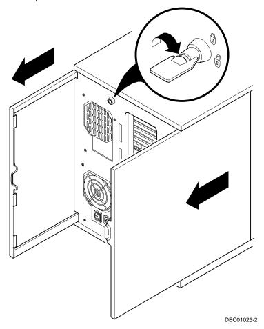
Figure 3-2. Unlocking and Removing the Side Panels
