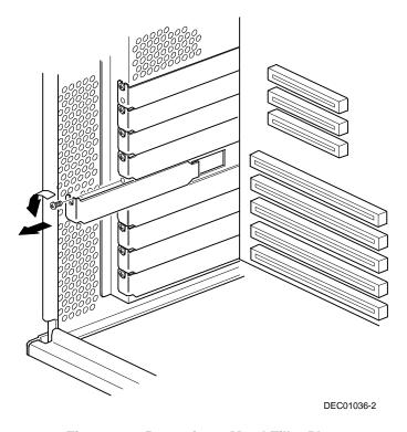
Figure 8-3. Removing a Metal Filler Plate
