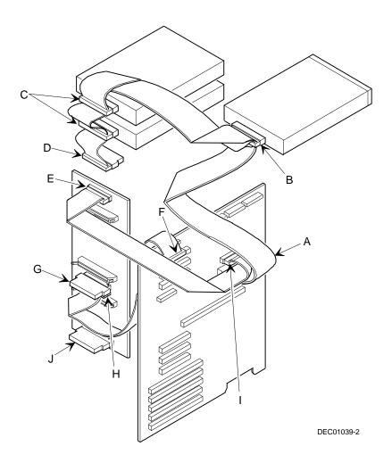
Figure 9-2. Split Backplane Using Onboard SCSI Controllers Configuration
