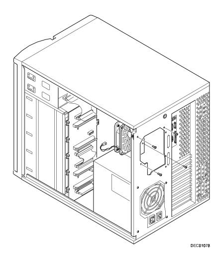
Figure 12-6. Removing and Replacing Cooling Fan 5
