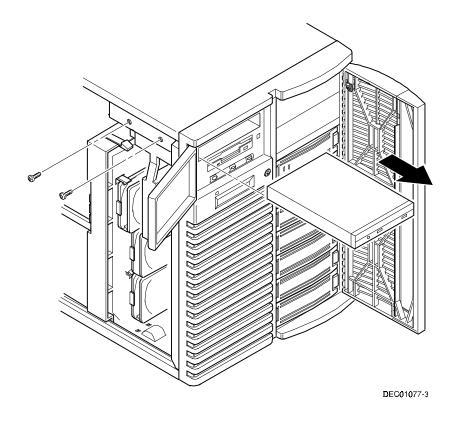
Figure 12-3. Removing and Replacing the CD-ROM Drive
