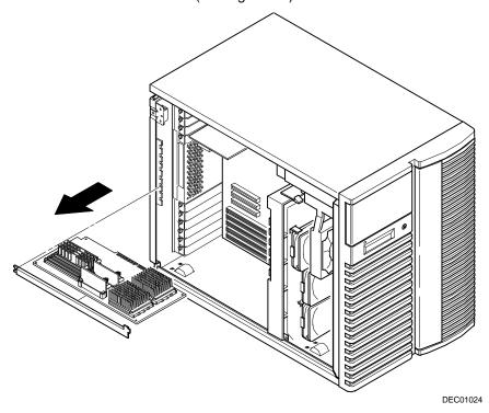
Figure 5-2. Removing the CPU Module
