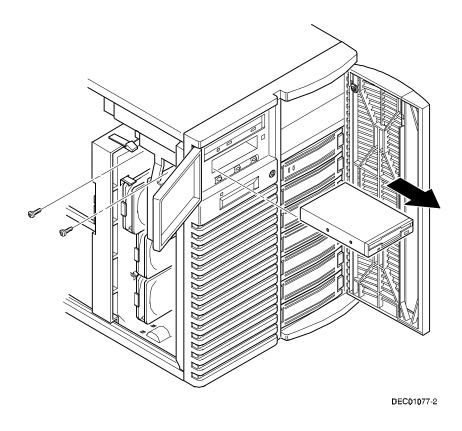
Figure 12-2. Removing and Replacing the Diskette Drive
