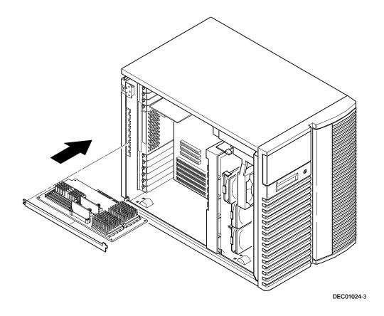
Figure 5-5. Installing a CPU Module
