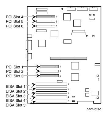
Figure 8-1. Expansion Board Slot Locations
