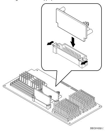
Figure 5-4. Installing the Regulators
