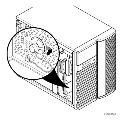
Figure 12-7. Removing and Replacing the Speaker
