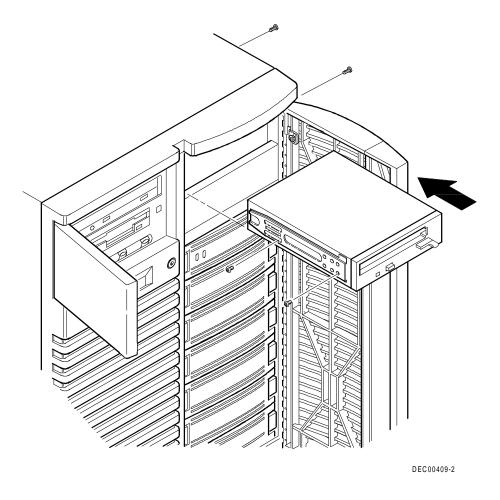
Figure 7-2. Installing a Half-Height 51/4-Inch Device Into Top-Right Drive Bay
