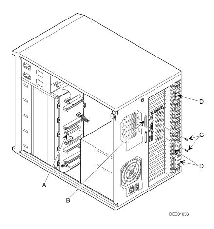
Figure 7-6. External SCSI Bus Connections
