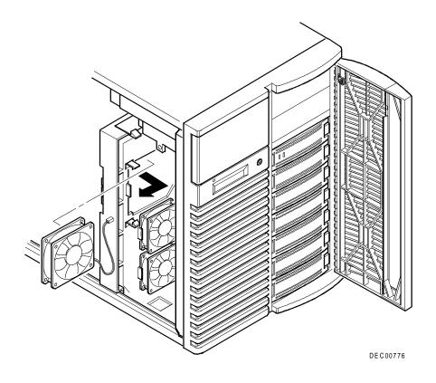
Figure 12-4. Removing and Replacing a Cooling Fan
