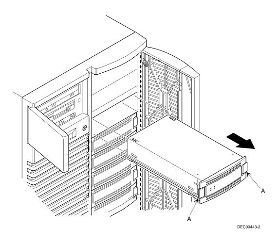
Figure 7-5. Installing a Device Into the Hot-Swap Drive Bay
