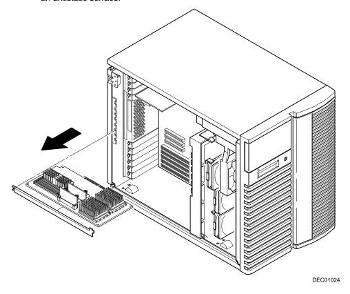
Figure 6-2. CPU Module Removal
