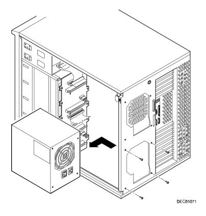
Figure 12-1. Removing and Replacing the Power Supply
