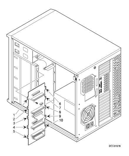
Figure 12-9. Removing and Replacing the Storage Backplane
