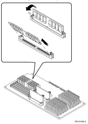
Figure 5-3. Removing SIMMs
