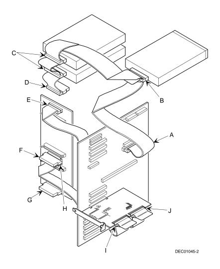
Figure 9-3. Split Backplane Using Two-Channel RAID Controller Configuration
