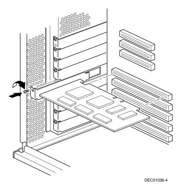
Figure 8-5. Installing an EISA Expansion Board
