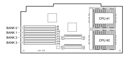
Figure 6-1. CPU Module SIMM Bank Locations
