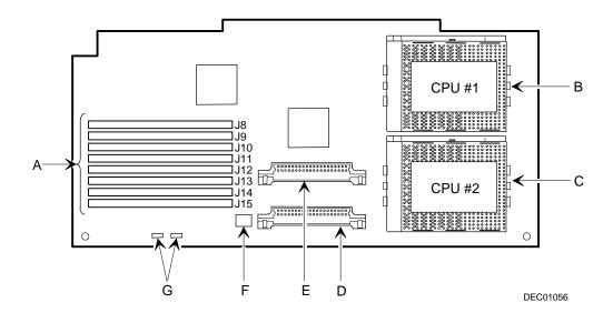
Figure 3-10. CPU Module Components and Connectors
