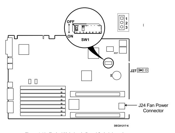
Figure 1-12. Typical Main Logic Board Switch Location
