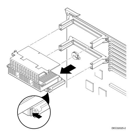
Figure 1-1. Releasing the Installed Processor
