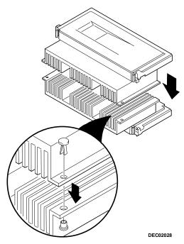
Figure 1-7. Attaching the New Processor
