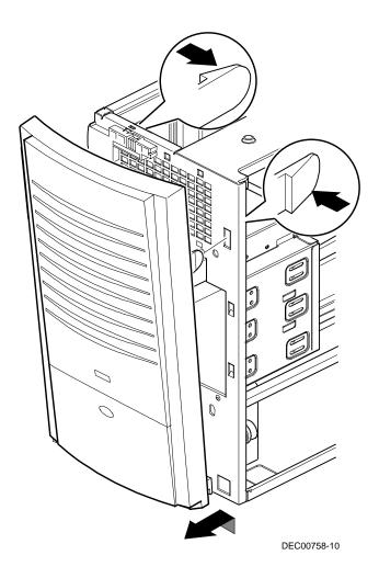
Figure 1-13. Removing the Front Bezel
