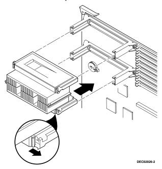
Figure 1-8. Installing Both Processors
