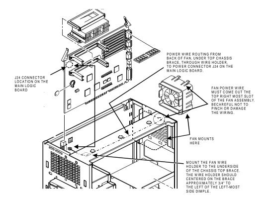
Figure 1-11. Wiring Path for additional Fan Assembly
