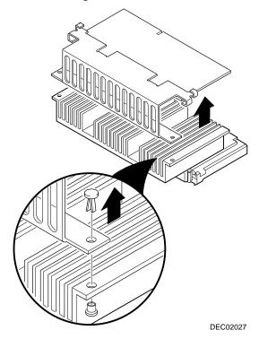
Figure 1-2. Removing the Bracket and Termination Card
