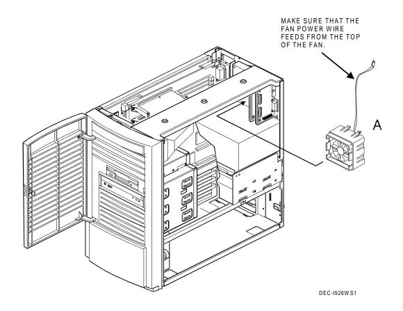
Figure 1-10. Installing the additional Fan Assembly
