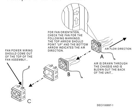
Figure 1-9. Installing the additional Fan Assembly
