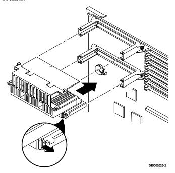
Figure 1-4. Reinstalling the Processor
