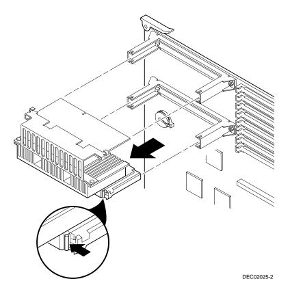
Figure 1-5. Releasing the Installed Processor
