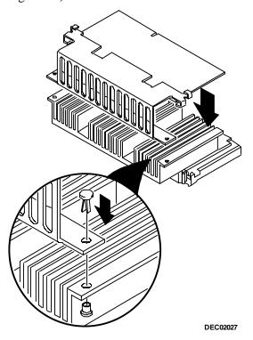
Figure 1-3. Installing the Bracket and Termination Card
