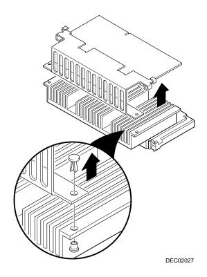
Figure 1-6. Removing the Bracket and Termination Card
