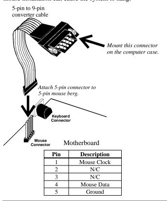
When connecting chassis connectors to the motherboard, make sure to connect the correct connector end. Most connector wires are color-coded. Match the color of the wires leaving the switch or LED to the same pin on the connector end. There may be more than one connector with the same colorcoded wires. If so, follow the wire to the switch or LED. Pin 1 is always indicated on the motherboard.
