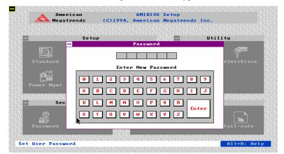
As shown on the above screen, you are prompted for a 1-6 character password. You can either type the password on the keyboard or select each letter of the password, one at a time, using the mouse. The password does not appear on the screen when typed. Make sure you write it down. If you forget it, you must drain NVRAM and reconfigure.
