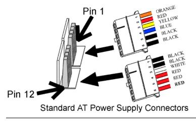
**Connector Keys** The keys on the connector must be cut to fit on some power supplies, as shown below.
