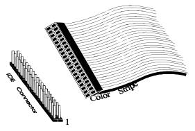
PRIMARY is a 40-pin dual-inline berg that connects an IDE drive to the primary onboard IDE connector. This motherboard supports IDE Modes 0, 1, 2, 3, and 4, IDE prefetch, LBA (Logical Block Address) mode, high capacity drives (over 528 MB), 32-bit data transfer, and fast IDE transfer. These IDE features are configured in Peripheral Setup in the WINBIOS Setup utility. Disable the onboard IDE interface in Peripheral Setup to use an ISA ESDI, RLL, MFM, or SCSI hard disk drive controller.
