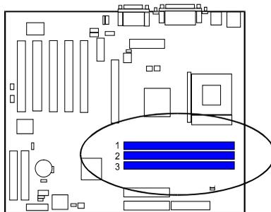
Press the clips with both hands to remove the DIMM.
