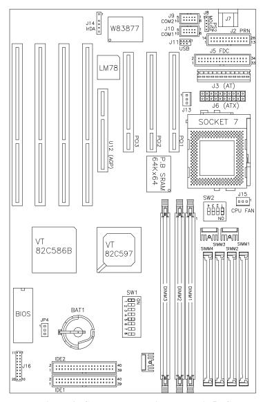
Figure 3: Connector Location on the AI5VG
