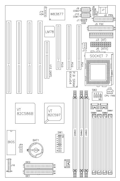
Figure 2: Jumper Locations of the AI5VG
