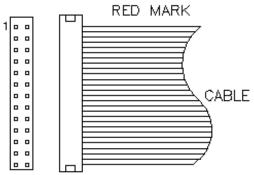
Figure 4: Orientation of the I/O Connector
