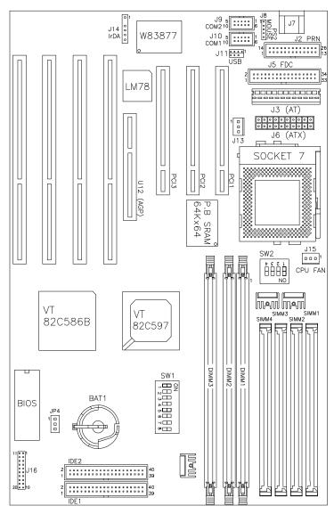
Figure 1: Layout of the AI5VG Motherboard
