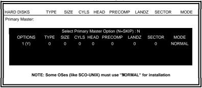
Up to four IDE drives can be detected, with parameters for each appearing in sequence inside a box. To accept the displayed entries, press the "Y" key; to skip to the next drive, press the "N" key. If you accept the values, the parameters will appear listed beside the drive letter on the screen.
