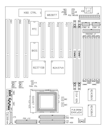
**Figure 3: Connector Location of the AI5TV**
