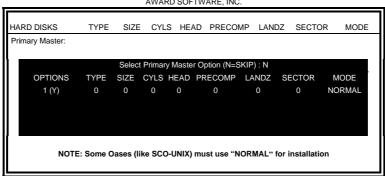
Up to four IDE drives can be detected, with parameters for each appearing in sequence inside a box. To accept the displayed entries, press the "Y" key; to skip to the next drive, press the "N" key. If you accept the values, the parameters will appear listed beside the drive letter on the screen.
