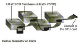
**NOTE:** Internal Ultra2 SCSI peripherals come from the factory with termination disabled and cannot be changed. Proper termination is provided by the built-in terminator at the end of the Ultra2 internal SCSI cable provided in the kit.
