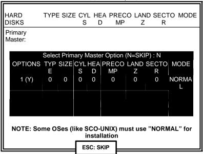
Up to four IDE drives can be detected, with parameters for each appearing in sequence inside a box. To accept the displayed entries, press the "Y" key to skip to the next drive, press the "N" key. If you accept the values, the parameters will appear listed beside the drive letter on the screen.
