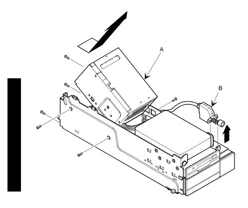
Figure 3 - 11 Removing the on Power Supply
