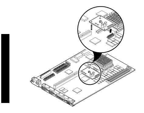
Figure 3 - 17 Installing the CPU Voltage Regulator
