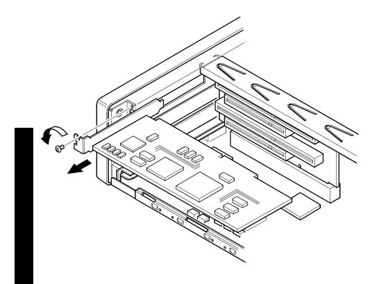
Figure 3 - 13 Removing Expansion Boards
