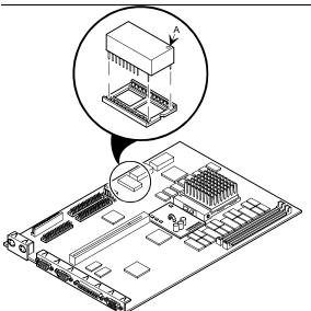
Figure 3 - 18 Replacing the Real Time Clock
