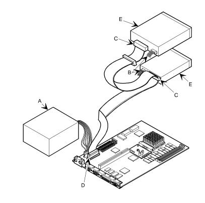
Figure 3 - 19 Diskette Drive Data Cable Connections
