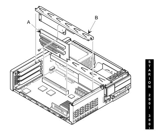
Figure 3 - 12 Removing the Riser Card & Bracket
