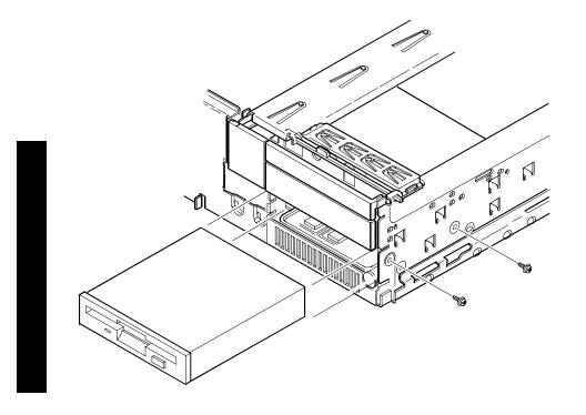
Figure 3 - 10 Removing the 3½-Inch Diskette Drive
