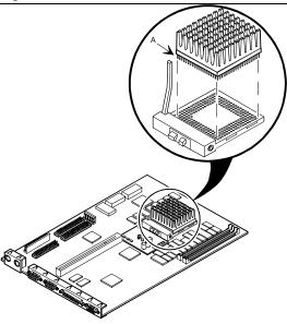
Figure 3 - 16 Installing a Higher Performance CPU
