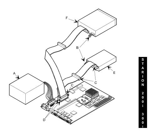
Figure 3 - 20 IDE Drive Data Cable Connections
