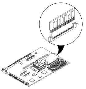
Figure 3 - 15 Installing External Cache Memory
