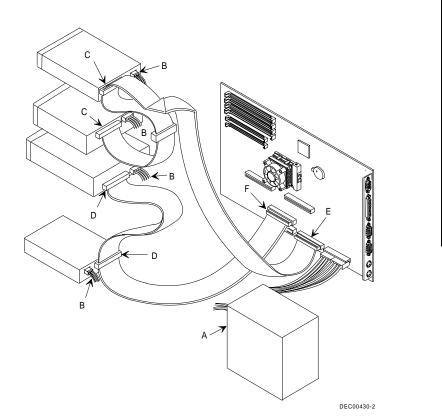
Figure 3 - 20 Diskette and IDE Data Cable Connections
