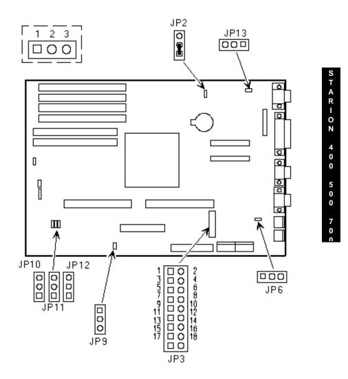
Figure 3 - 4 STARION 400/500 Main Logic Board Jumper Locations
