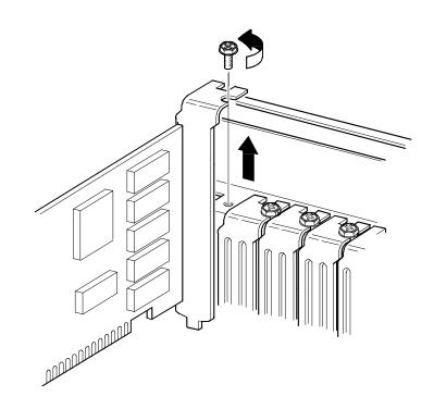
Figure 3 - 11 Removing Expansion Boards
