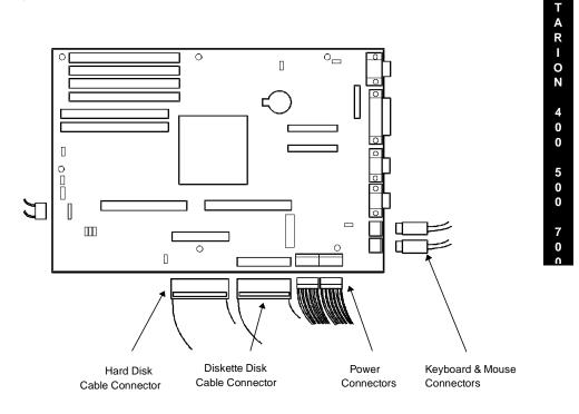
Figure 3 - 12 Removing the Main Logic Board (STARION 400/500 shown)
