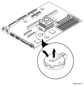
Figure 3 - 19 Replacing the Computer Battery
