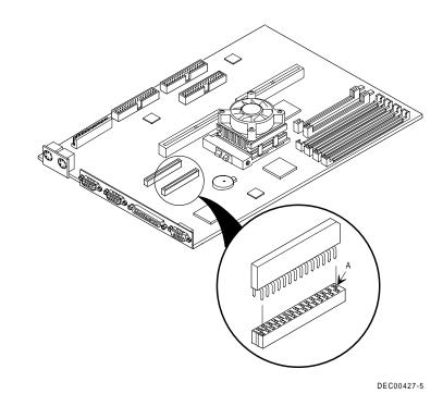
Figure 3 - 17 Installing Video Memory on the STARION 400/500
