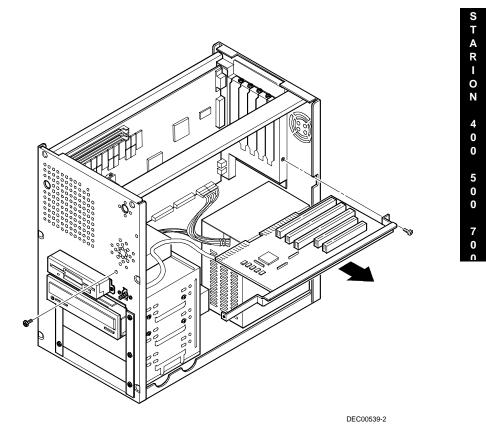
Figure 3 - 14 Removing Riser Card & Bracket
