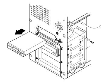
Figure 3 - 8 Removing the 3½-Inch Diskette Drive
