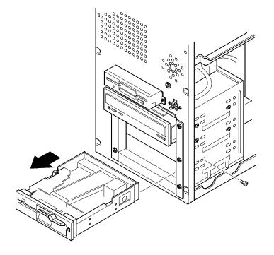
Figure 3 - 9 Removing a 5<sup>1</sup>/<sub>4</sub>-Inch Device
