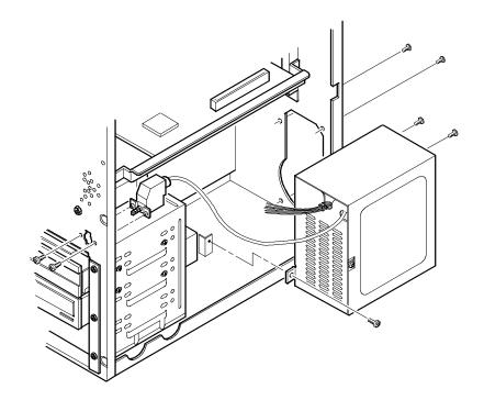
Figure 3 - 13 Removing the Power Supply
