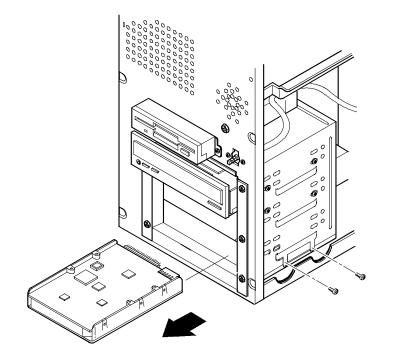
Figure 3 - 10 Removing the IDE Hard Disk Drive
