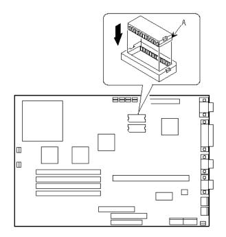
Figure 3 - 18 Installing Video Memory on the STARION 700
