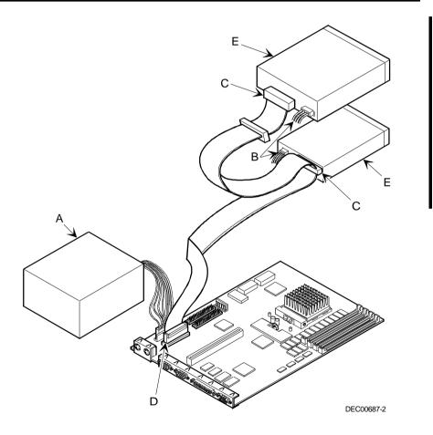
Figure 3 - 26 Diskette Drive Data Cable Connections
