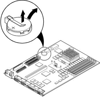
Figure 3 - 25 Replacing the Lithium Battery
