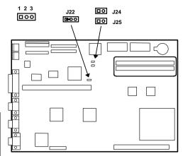
Figure 3 - 8 VENTURIS 560 Main Logic Board Jumpers Locations
