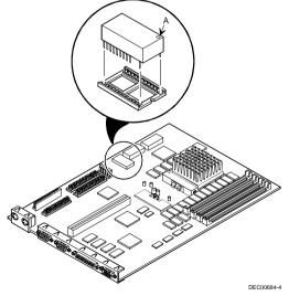
Figure 3 - 24 Replacing the Real-Time Clock
