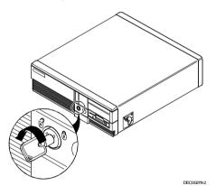
Figure 3 - 1 Unlocking the Cover
