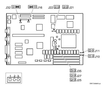
Figure 3 - 10 VENTURIS Pentium version 2.0 Main Logic Board Jumper Locations
