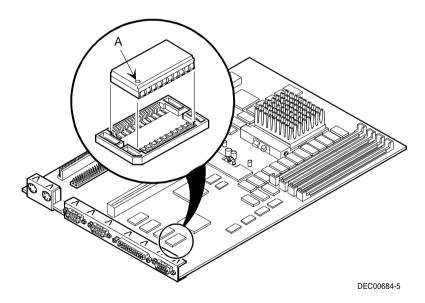
Figure 3 - 23 Installing Video Memory
