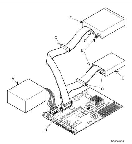
Figure 3 - 27 IDE Data Cable Connections
