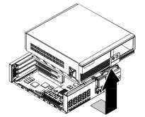
Figure 3 - 3 Removing the Cover
