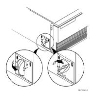
Figure 3 - 2 Releasing the Cover
