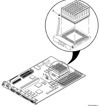
Figure 3 - 22 Installing a Higher Performance CPU
