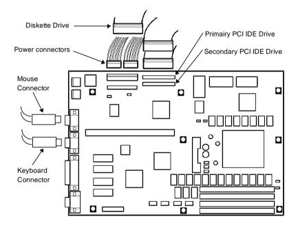
Figure 3 - 19 Removing the VENTURIS Pentium Main Logic Board
