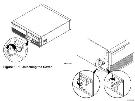
Figure 3 - 2 Releasing the Cover
