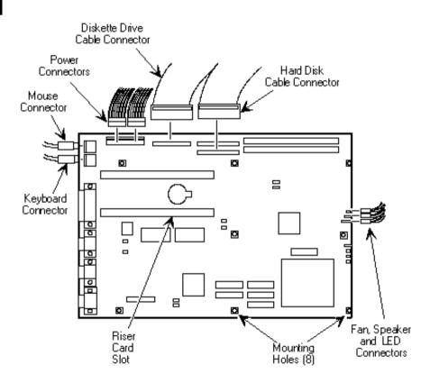
Figure 3 - 17 Removing the VENTURIS 486 Main Logic Board
