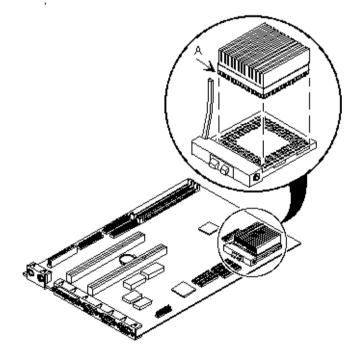
Figure 3 - 24 Installing a Higher Performance CPU on the VENTURIS 486 models
