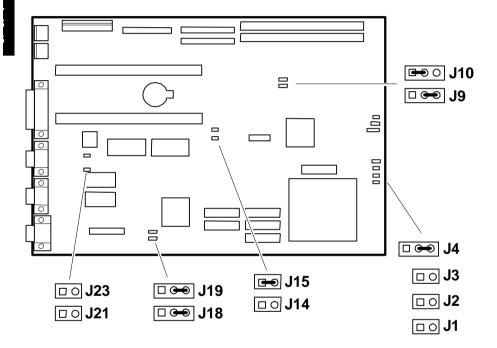
Figure 3 - 8 VENTURIS 486 version 1.0 Main Logic Board Jumpers Locations
