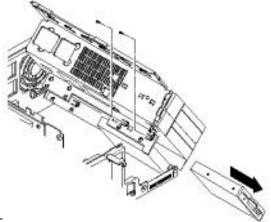
Figure 3 - 16 Removing the 3½-inch Diskette Drive on the VENTURIS 486 Full-Profile models
