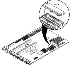
Figure 3 - 23 Installing External Cache Memory on the VENTURIS 486 version 2.0 board
